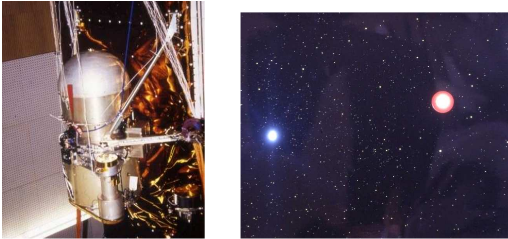
Fig. 9. (left) The UK Wide Field Camera which flew piggy back on ROSAT. (right) First EUV detection identified as a red dwarf - white dwarf binary system (from BBC Sky at Night)
